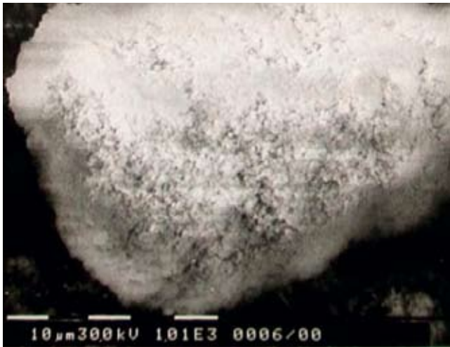
1 Calcium hydroxide particle • Kalkhydratpartikel
